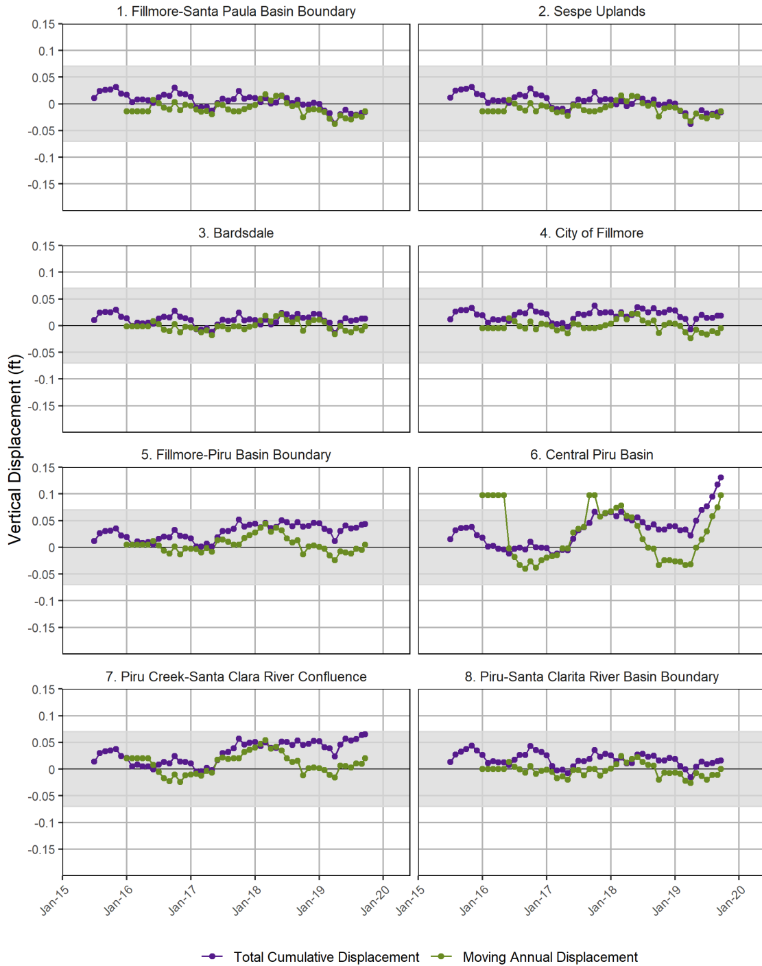
Figure 7: Time-series graphs showing running annual and total land surface elevation changes derived from InSAR data processed by TRE for select points in the basins.
