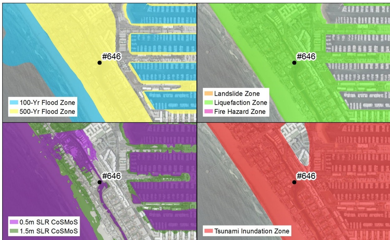
Figure 1. Hazard Zones for Venice Pumping Plant No. 646
