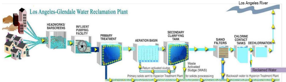
Figure 10 Treatment Process for the Los Angeles-Glendale WRP
