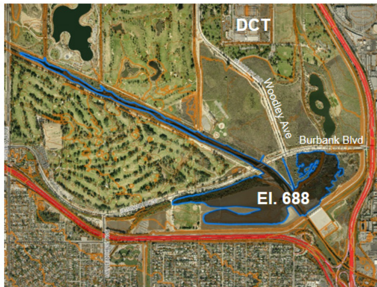
Figure 4: Inundation Area at El. 688 Upstream of Sepulveda Dam
