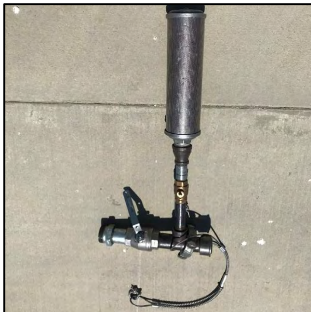
Figure IV Airlift control manifold (airhead). The airhead is used to control the delivery of high-pressure air from the air compressor into the well through the air-line.
