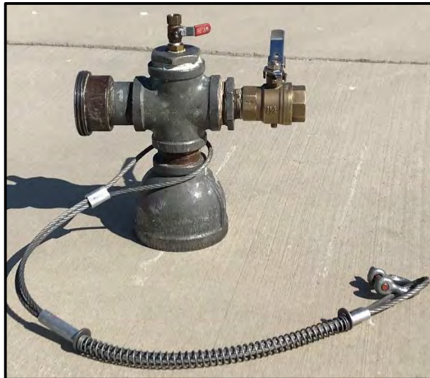
Figure V Image of 4-inch by 2-inch reducer/tee. When using the 3-inch camera tube as an airline, this Reducer/tee is used to connect the camera tube (air-line) to the airhead.
