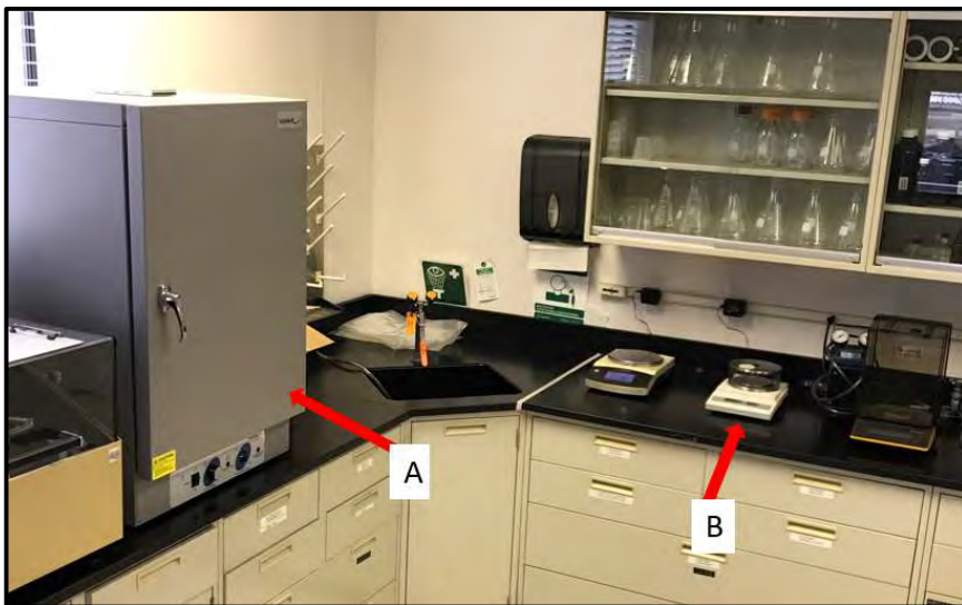
Area 145 Research Center Laboratory. Filter elements are dried in the oven (A) and weighed on the scale (B).
