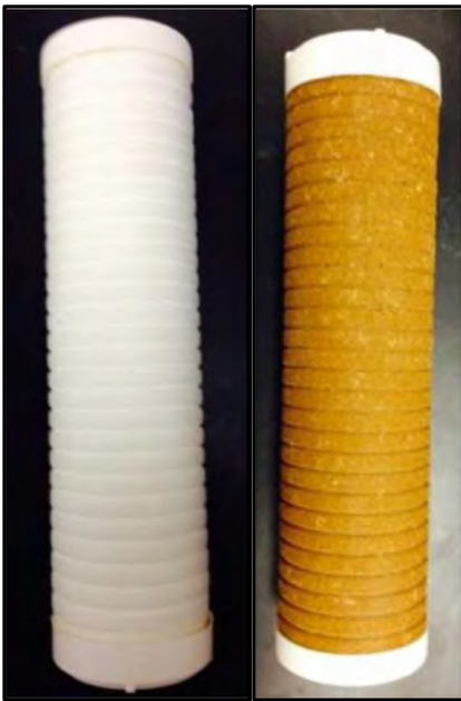
Figure 15 (B) Inside the blue filter housing (Figure 15 (A)) are the 1 and 5 micron filter elements. A new 1 micron filter element is shown on the left and a loaded 1 micron filter element after 1 month of service is shown on the right. The filters are weighed and the difference in weight is mathematically extrapolated to determine the mass loading of the injection wells. The red color is thought to be the result of iron oxidation occurring at the GWRS treatment plant.
