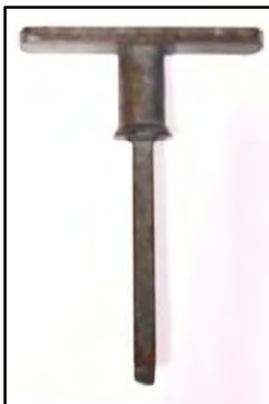
Figure 21 Hand tool (“T-handle”) used to open Legacy Well Vault manway hatch.
