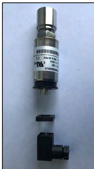
Figure 28 Legacy Well pressure indicating transmitter assembly. Pressure sensing device (top), gasket (middle) and plug (bottom). The plug rarely fails. Gaskets should be changes when replacing the pressure sensing devise. This is a low voltage assembly. The warehouse stocks these parts.
