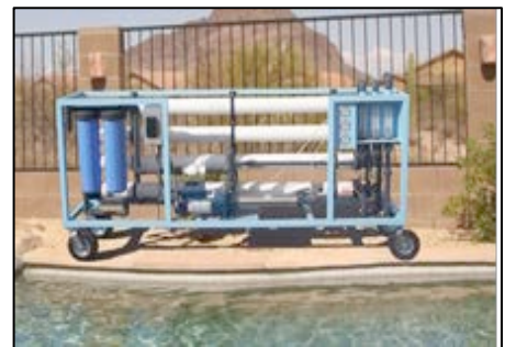
Figure 7.62 - Pool Reverse Osmosis System
