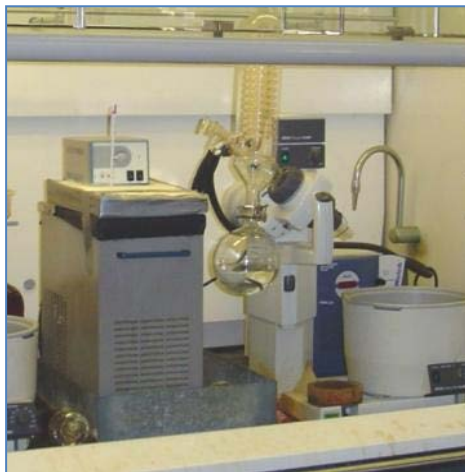
Figure 7.55 - Recirculating Refrigeration System in a Chemistry Laboratory
