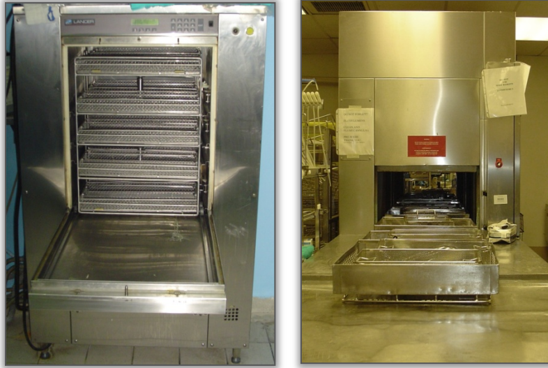
Figure 7.18 - Batch and Conveyor (Tunnel) Washer - Disinfectors in Central Sterile Operations
