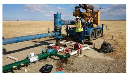
Figure ES-3. Wellhead Control and Other Equipment
