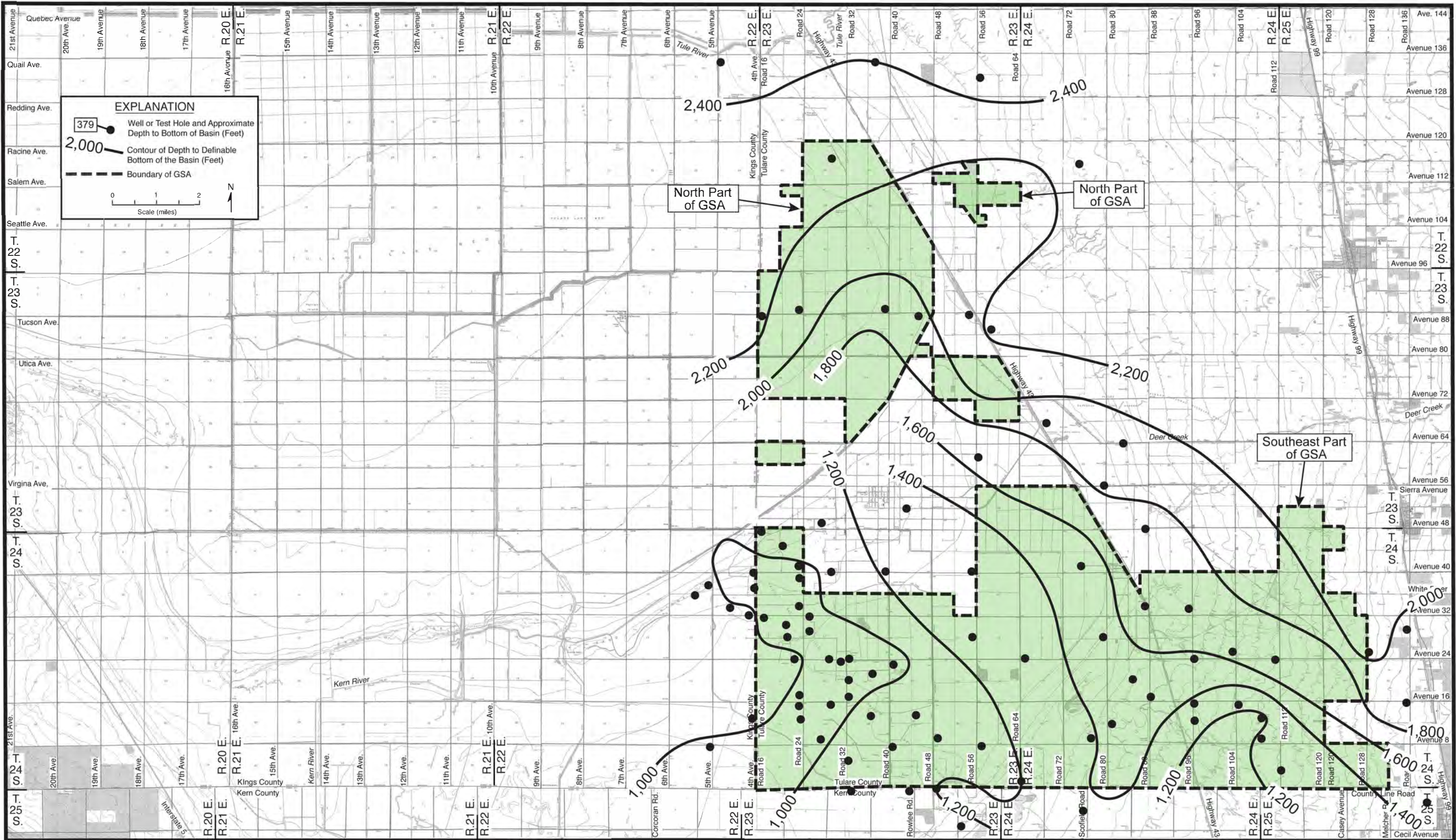
FIGURE 2.1.1 - DEFINABLE BOTTOM OF THE BASIN
