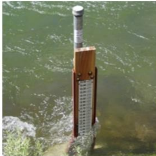
Figure 6 – Simple Stilling Well and Staff Gage Setup
