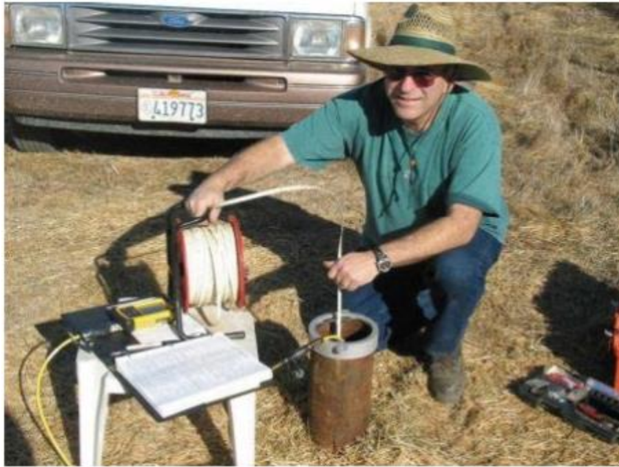
Figure 3 – Collection of Water Level Measurement and Pressure Transducer Download
