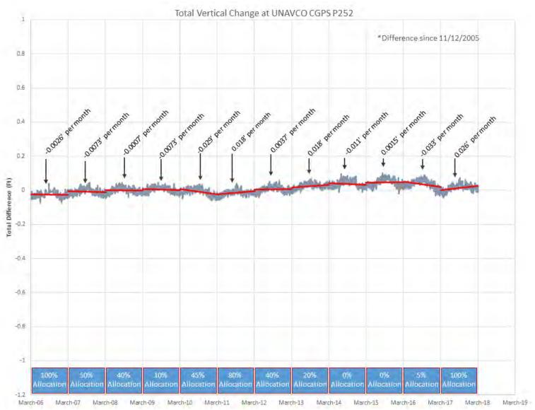
Figure 5-109. Vertical Elevation Change at UNAVCO CGPS P252, Spring 2006 to 2018
