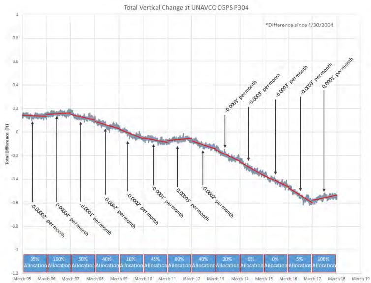
Figure 5-112. Vertical Elevation Change at UNAVCO CGPS P304, Spring 2005 to 2018
