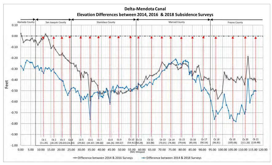
Figure 5-117. Elevation Change along the Delta-Mendota Canal, 2014 through 2018
