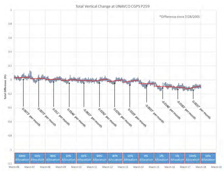
Figure 5-108. Vertical Elevation Change at UNAVCO CGPS P259, Spring 2006 to 2018
