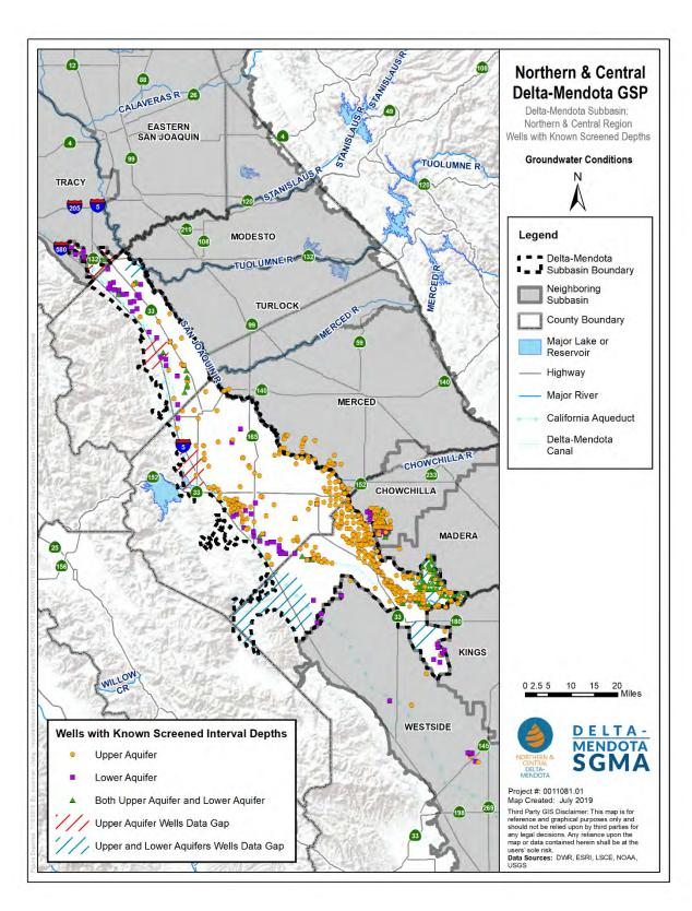
Figure 5-64. Wells with Known Screened Interval Depths, Delta-Mendota Subbasin
