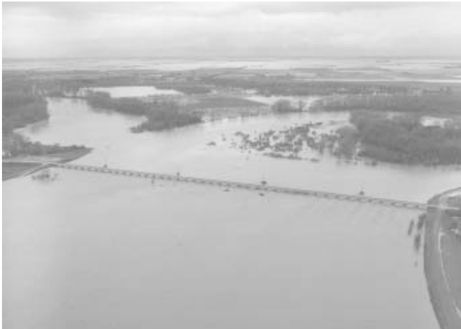
Overflow at Colusa Weir on March 11, 1995. The Colusa Basin is the flooded area in the background.
