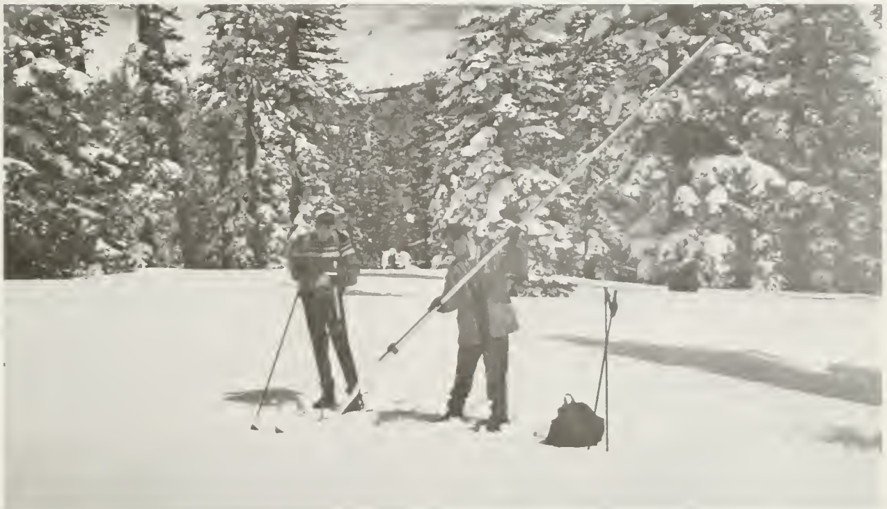
MEASURING THE RECORD WATER CONTENT--Two snow surveyors from the Department of Water Resources measure the water content of a 140-inch snowpack at Wrights Lake in the American River drainage basin. The snow core picked up in the tube contained 67 inches of water, contrasted to the 50-year average of 33 inches for April 1. The snow course is at an elevation of 6,900 feet in the Sierra Nevada. Pyramid Peak appears between the trees in the background.
