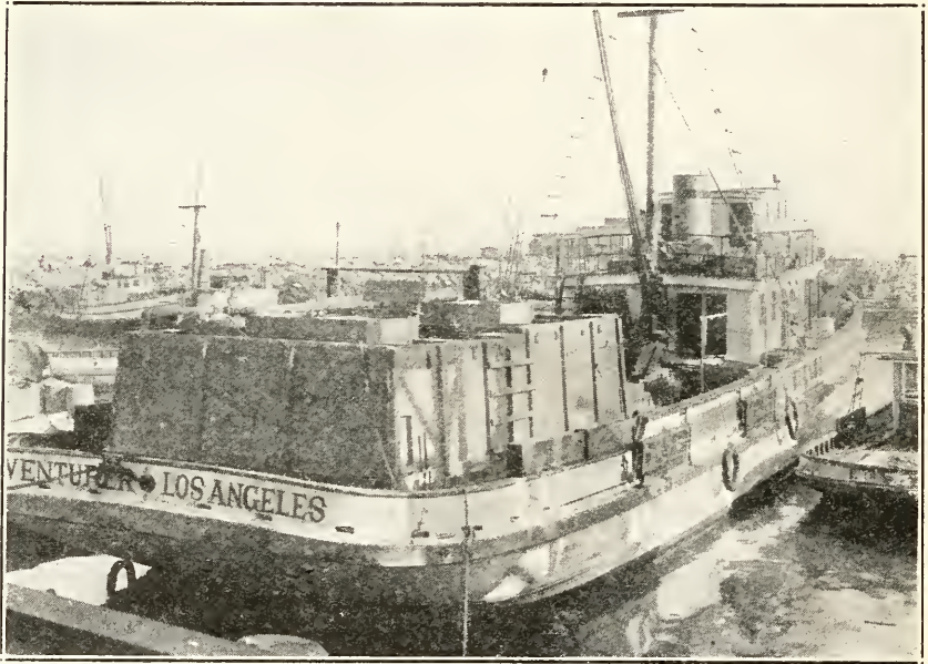
FIG. 36. New type of fishing boat used off Mexican coast. Several tons of live bait carried in tanks have given this type the name of "bait boat." Photograph by E. S. Cheney.
