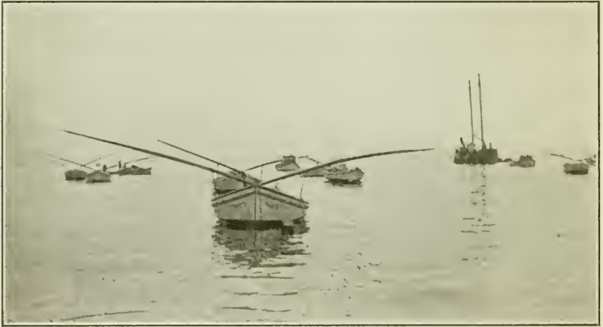
Fig. 13. Salmon boat on Monterey Bay with outriggers for trolling. Photograph by N. B. Scofield.
