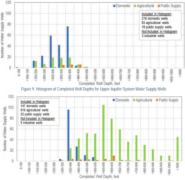
Figure 10. Histogram of Completed Well Depths for Lower Aquifer System Water Supply Wells
