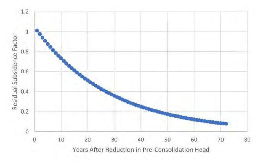
Figure 5. Residual Subsidence Factors for Years After Reduction in Pre-Consolidated Head
