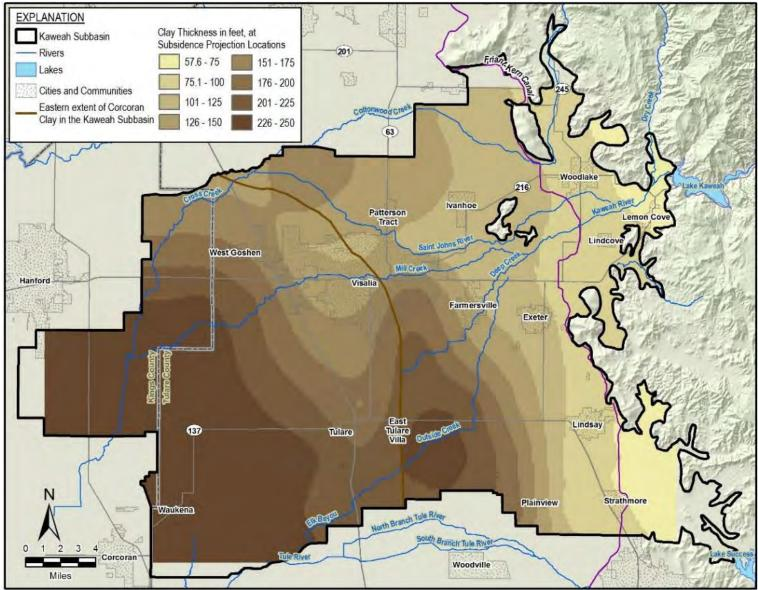
Figure 8. Clay Thickness from Spreadsheet Tool Calibration
