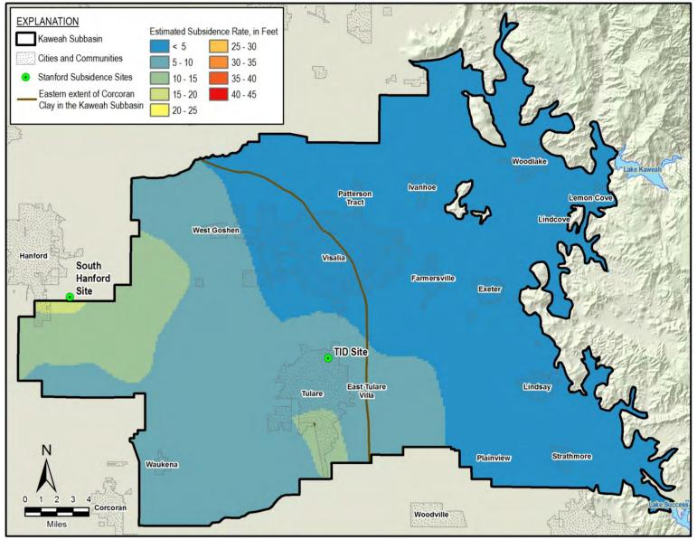
Figure 15. Spreadsheet Tool Estimated 2040 to 2070 Subsidence when Groundwater Levels Stabilize at Measaurable Objectives
