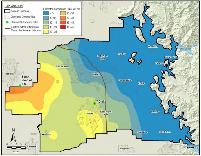
Figure 16. Spreadsheet Tool Estimated 2020 to 2070 Subsidence when Groundwater Levels Stabilize at Measaurable Objectives
