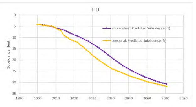
Figure 7. Spreadsheet and Model Predicted Subsidence at South Hanford and TID Sites, 1999-2070
