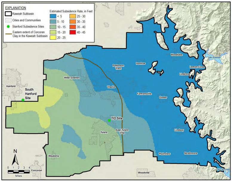
Figure 14. Spreadsheet Tool Estimated 2020 to 2040 Subsidence when Groundwater Levels Stabilize at Measaurable Objectives
