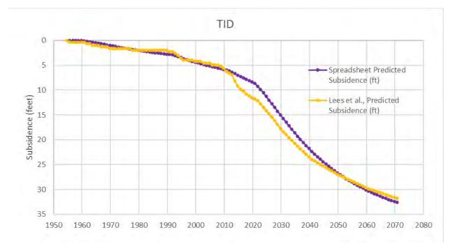
Figure 6. Spreadsheet and Model Predicted Subsidence at South Hanford and TID Sites, 1954-2070
