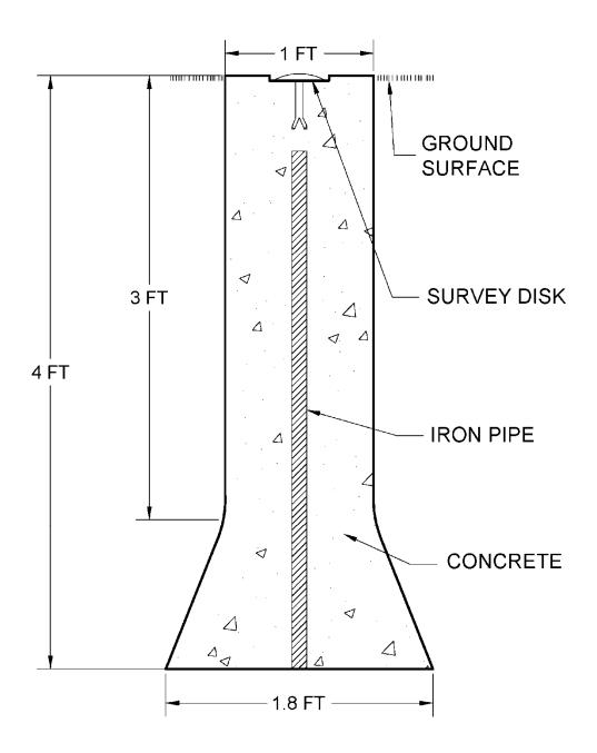
Figure 2 - Modified NGS Concrete Type Survey Monument
