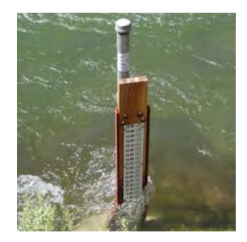
Figure 6 – Simple Stilling Well and Staff Gage Setup
