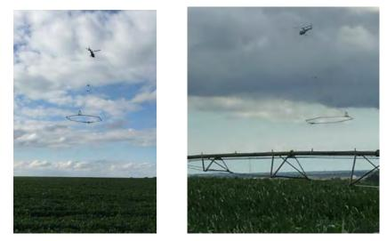
Figure 4-4: Photos of the SkyTEM312 system in suspension beneath the helicopter.
