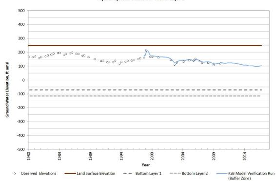
Well KSB-1535 Well ID: 21S24E03L01M Aquifer System: Upper - Model Layer 3 Total Depth (ft): 325
