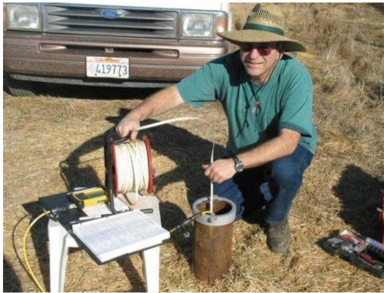
Figure 3 – Collection of Water Level Measurement and Pressure Transducer Download
