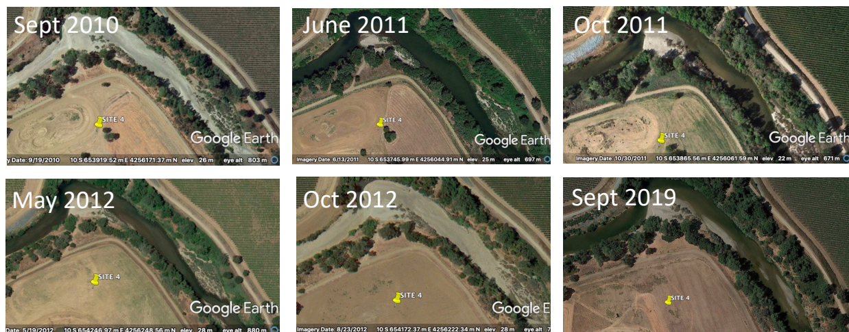
Figure 31: Selected dates of 30-centimeter pan-sharpened true color images of a selected location along the Cosumnes River qualitatively demonstrate the effectiveness high-resolution satellite imagery in determining drying events.
