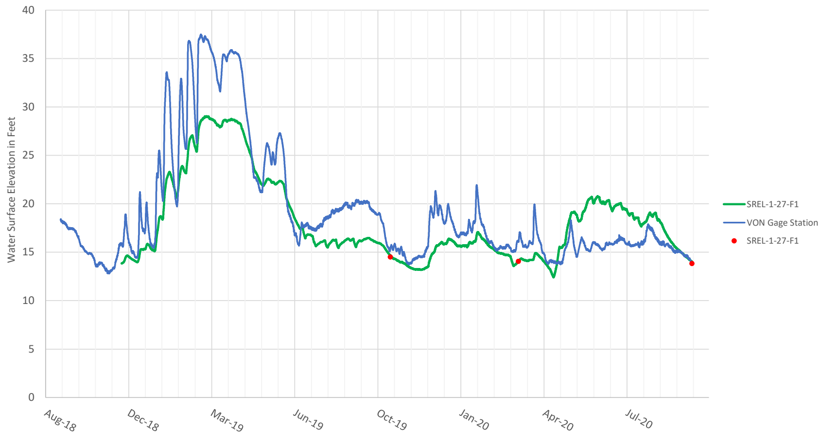
Surface Water/Groundwater Interaction - Sacramento River SREL-1-27-F1 Monitoring Well and Sacramento River Stage Hydrographs
