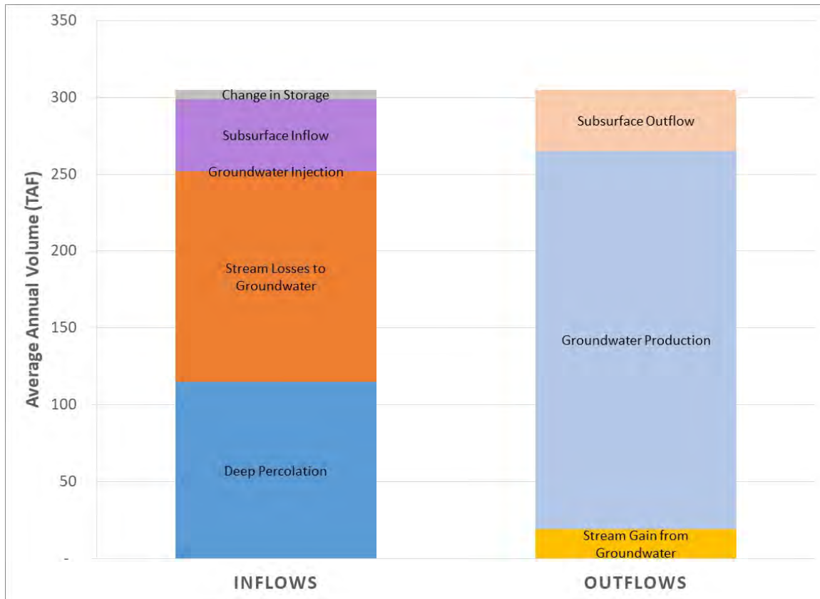
Figure 2.4-14: Projected Conditions With Climate Change Average Annual Water Budget – Groundwater System, South American Subbasin
