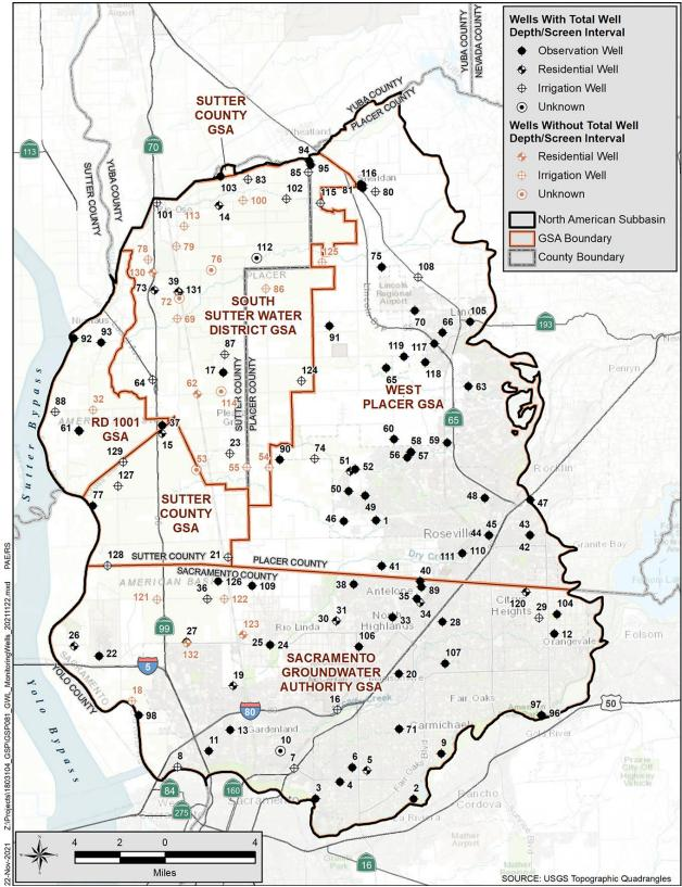
Figure 7-1. Groundwater Level Monitoring Network Wells
