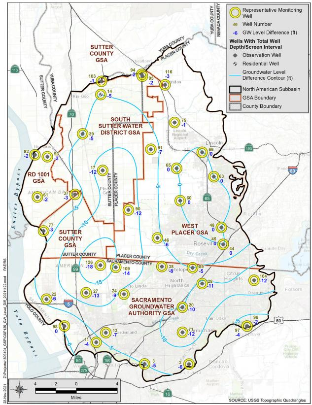
Figure 8-5. Projected Groundwater Elevation Changes at RMS Locations
