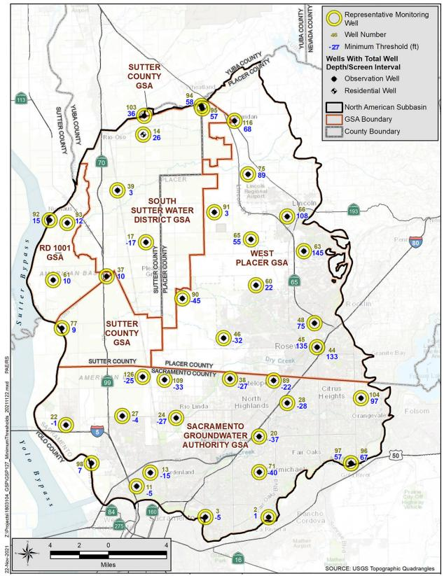
Figure 8-6. Projected Groundwater Elevation MTs at RMS Locations
