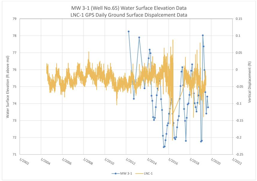
Figure 5-27. CGPS Station LCN1 versus Groundwater Levels
