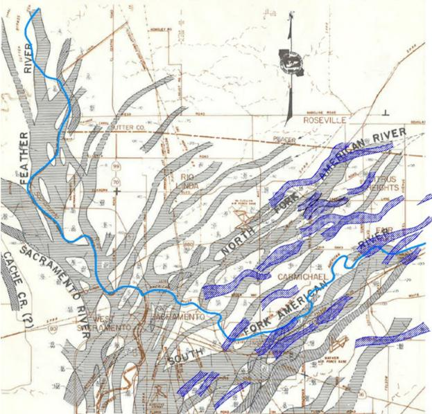
Figure 4-8. Stream Channel Deposits
