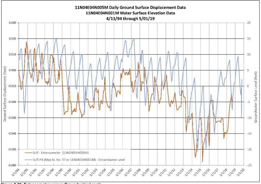
Figure 5-26. Extensometer versus Groundwater Levels
