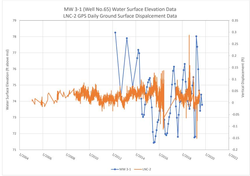
Figure 5-28. CGPS Station LCN2 versus Groundwater Levels
