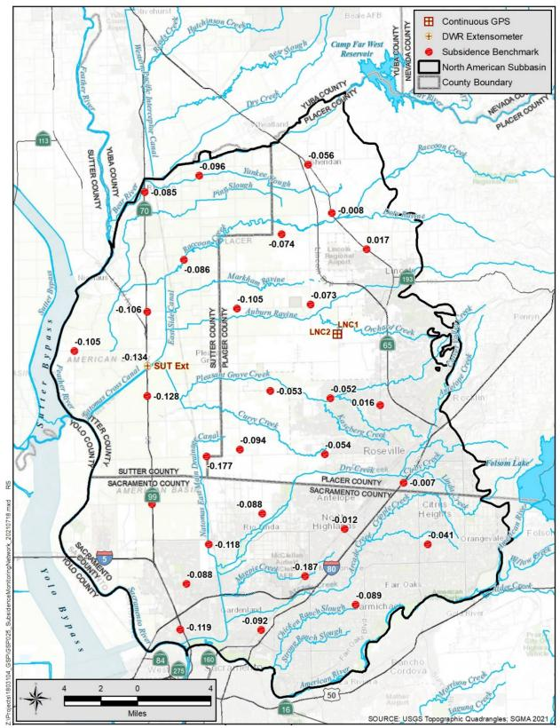
Figure 3-20. Subsidence Monitoring Network
