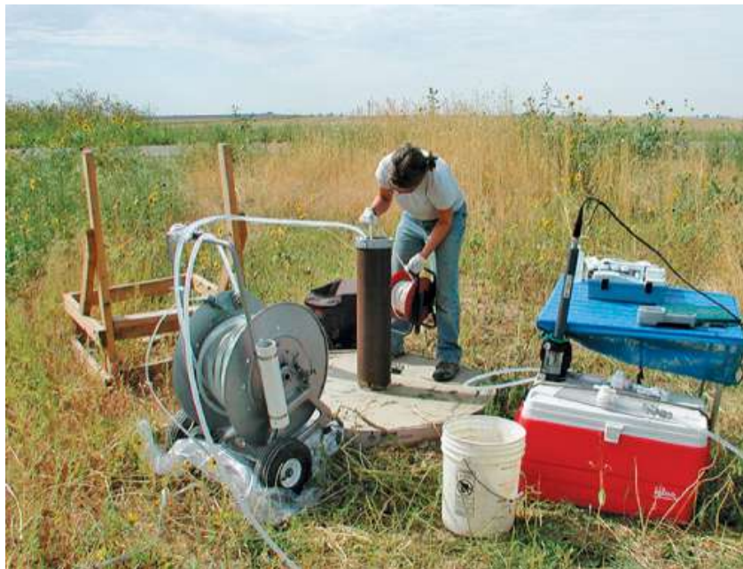
Figure 5 – Typical Groundwater Quality Sampling Event
