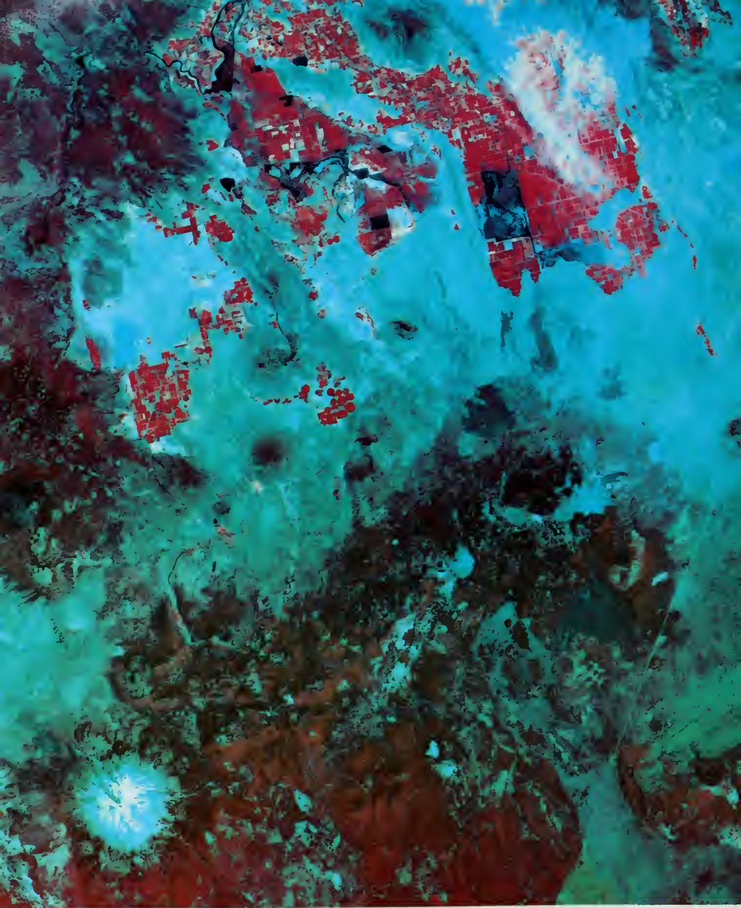
This Landsat satellite scene covers the area from Mt. Shasta on the south (lower left) to southern Oregon on the north. Irrigated lands appear as red areas. The circular red shapes at center are fields being irrigated by large center-pivot irrigation systems, which have become popular in northeastern California.
