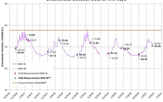
Groundwater Elevation Data for MW-9S/D
