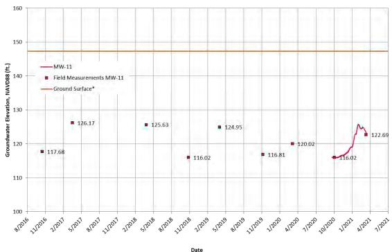
**Groundwater Elevation Data for MW-11**
