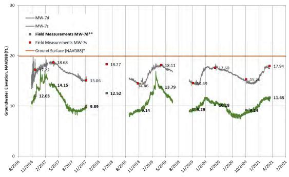
Groundwater Elevation Data for MW-7S/D
