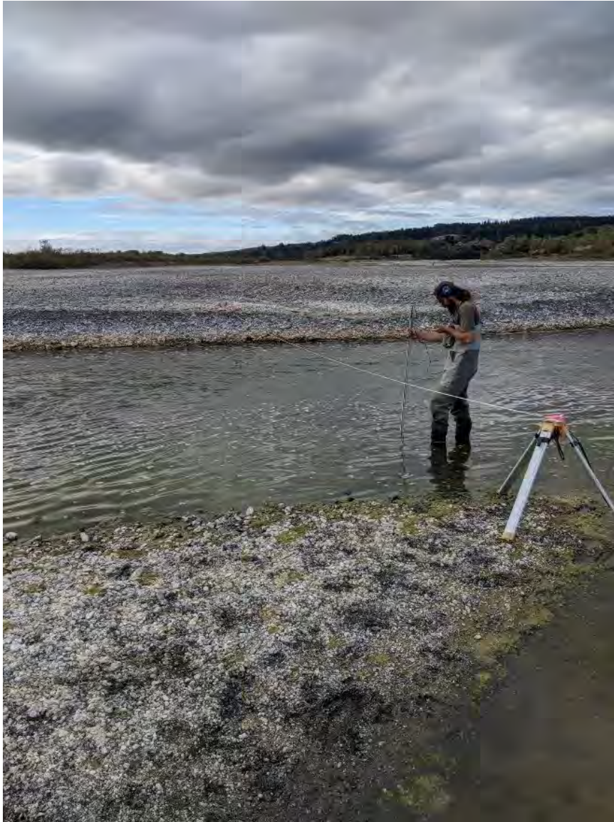
Figure 12. Streamflow measurement at QM-2
