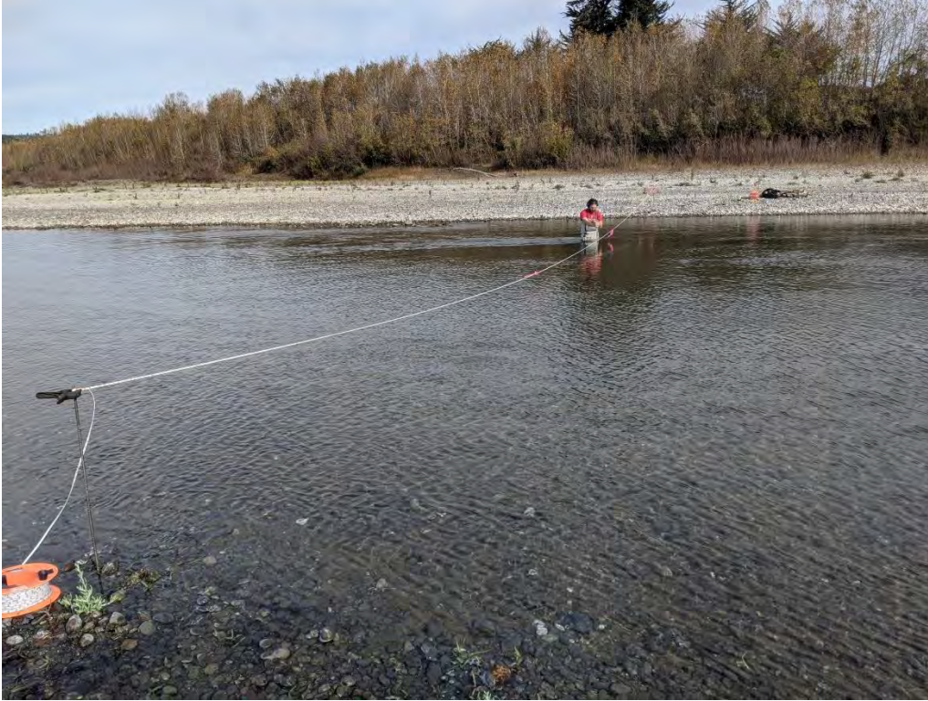
Figure 5. Discharge measurement below R-2
