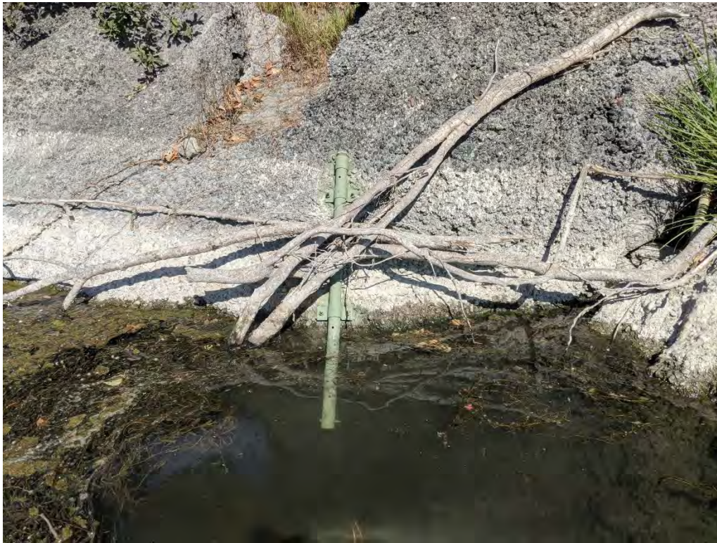
Figure 3. Gauge in housing at R-5. Additional vegetation was added later for increased camouflage.
