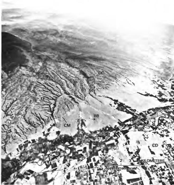
FIGURE 13.—Composite of two U.S. Air Force high-altitude oblique aerial photographs showing pronounced linear trace of Chico monocline (CM, upper right to lower left), broad alluvial fan west of Chico monocline capped by Red Bluff Formation (RB, gray, uncultivated grazing land), and dissected topography of Tuscan Formation (TF) to east. DC, Deer Creek; CD, north Corning dome. Sacramento River (SR) follows trace of Los Molinos syncline (LMS) between north Corning dome and alluvial fan to east.
