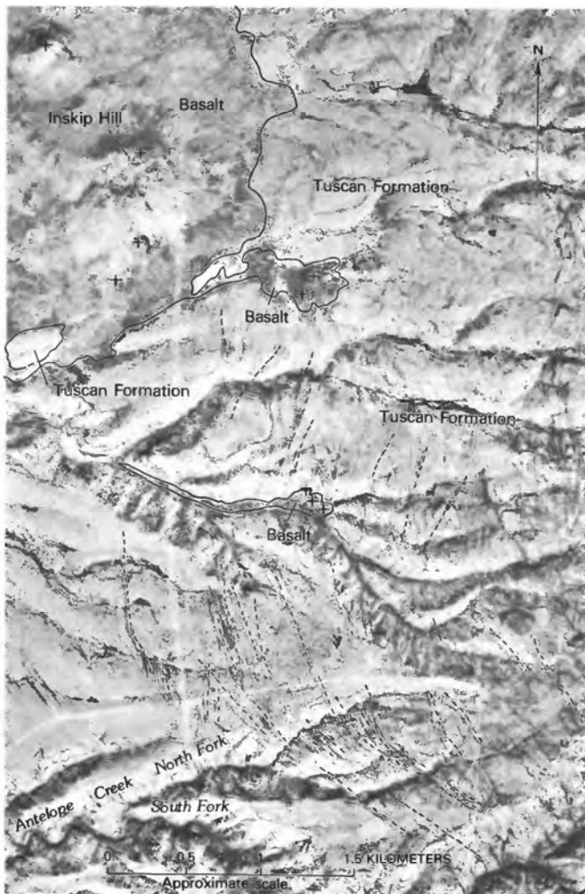
FIGURE 19.—Low-altitude vertical aerial photograph (U.S. Geological Survey) showing arcuate fault pattern (dashes) and cinder cones (crosses) south of Inskip Hill. Gray incised plains are underlain by the Tuscan Formation; thin dark lines are concentrations of brush and trees growing along fault traces.
