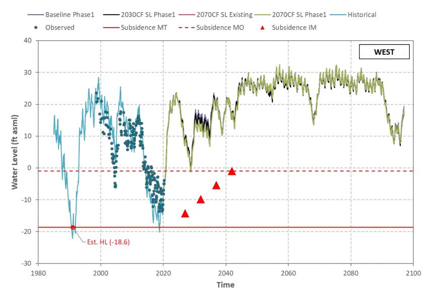
Figure I-21 Mugu Aquifer - Simulated/Observed Water Level (Well 02N23W15J02S).
