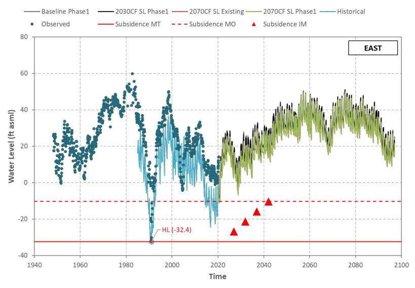
Figure I-3 Hueneme Aquifer - Simulated/Observed Water Level (Well 02N22W09K04S).
