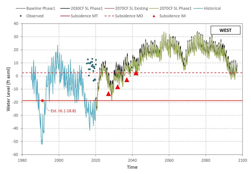
Figure I-10 Hueneme Aquifer - Simulated/Observed Water Level (Well 02N22W17M02S).
