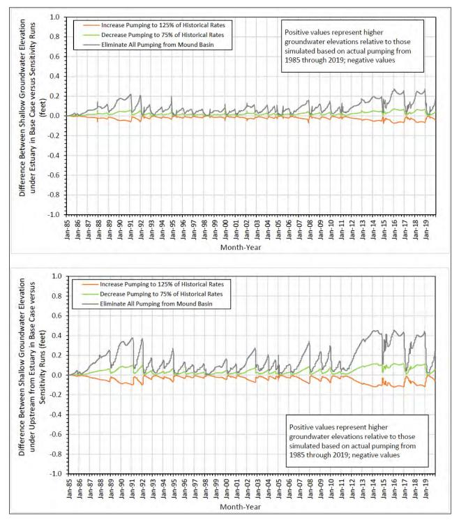
Figure G-10. Graphs Showing Differences Between Simulated Groundwater Elevations in Shallow Alluvial Deposits in Base-Case Scenario Compared to Sensitivity Runs under Santa Clara River estuary (top graph) and under Santa Clara River near Boundary between Mound and Oxnard Basins (bottom graph)
