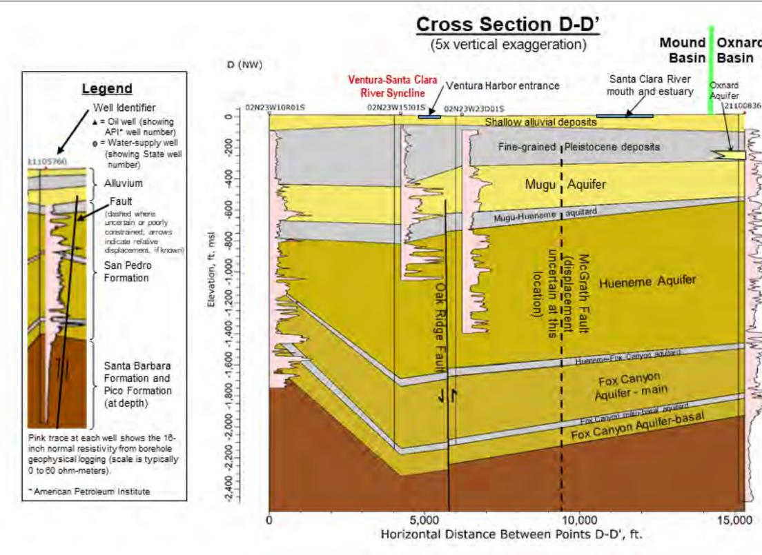
Figure G-6. Cross Section D-D' Showing Hydrostratigraphic Units below the Santa Clara River in Mound Basin (Figure 3.1-08 of the Draft Mound Basin GSP)
