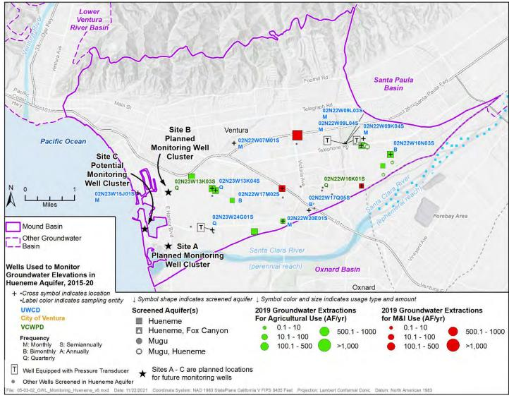
Figure I-2 Map Showing the Groundwater Elevation Monitoring Network in the Hueneme Aquifer of Mound Basin Aquifer of Mound Basin.
