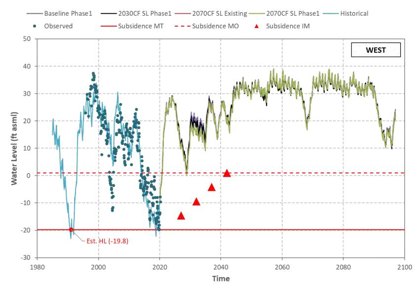
Figure I-18 Mugu Aquifer - Simulated/Observed Water Level (Well 02N22W07M02S).
