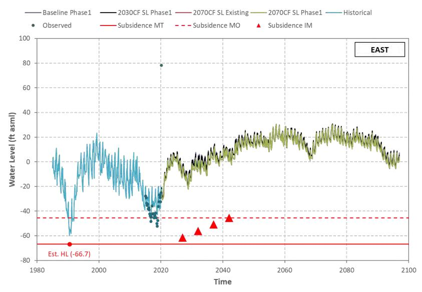
Figure I-8 Hueneme Aquifer - Simulated/Observed Water Level (Well 02N22W17Q05S).
