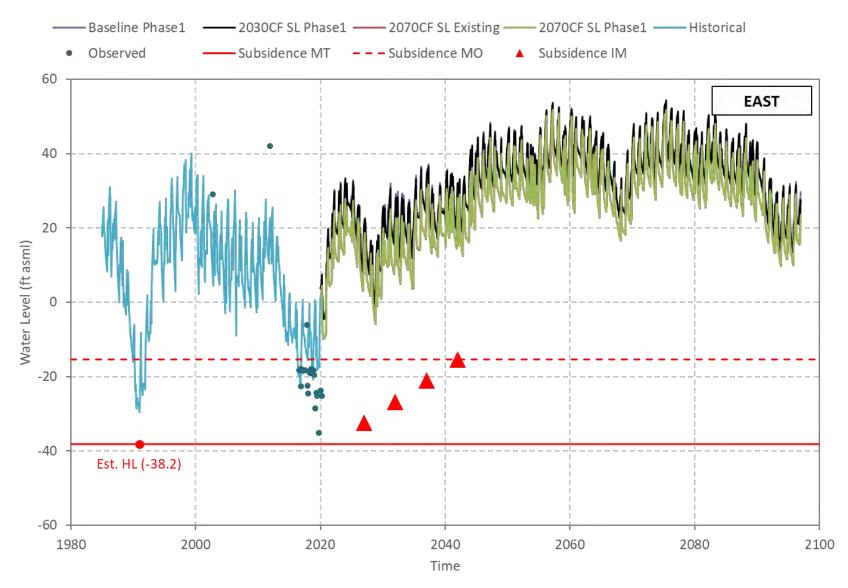
Figure I-6 Hueneme Aquifer - Simulated/Observed Water Level (Well 02N22W10N03S).
