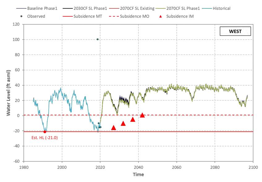
Figure I-19 Mugu Aquifer - Simulated/Observed Water Level (Well 02N22W07P01S).
