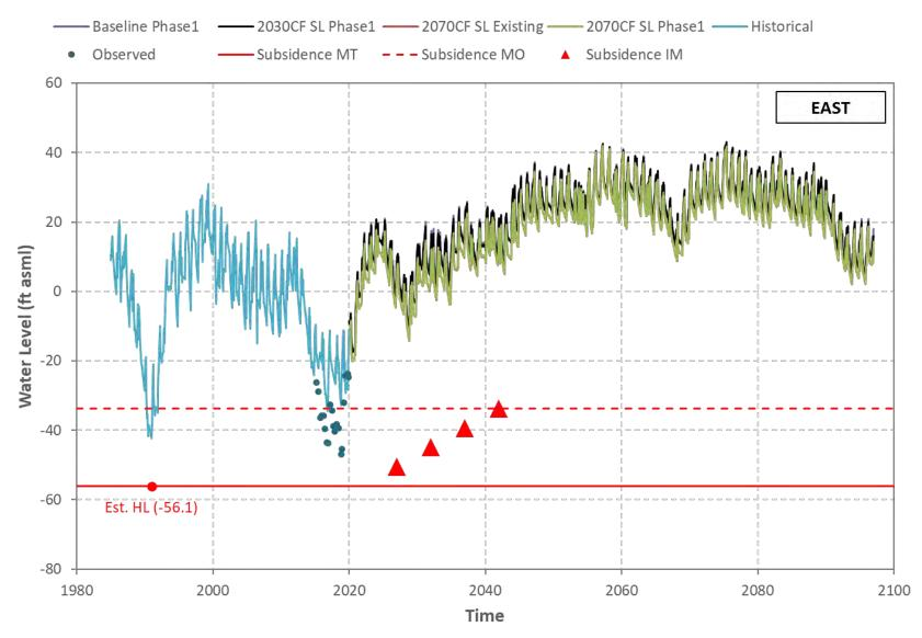
Figure I-7 Hueneme Aquifer - Simulated/Observed Water Level (Well 02N22W16K01S).
