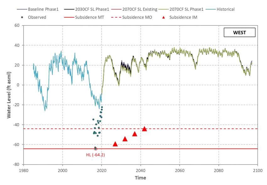
Figure I-20 Mugu Aquifer - Simulated/Observed Water Level (Well 02N22W19M04S).
