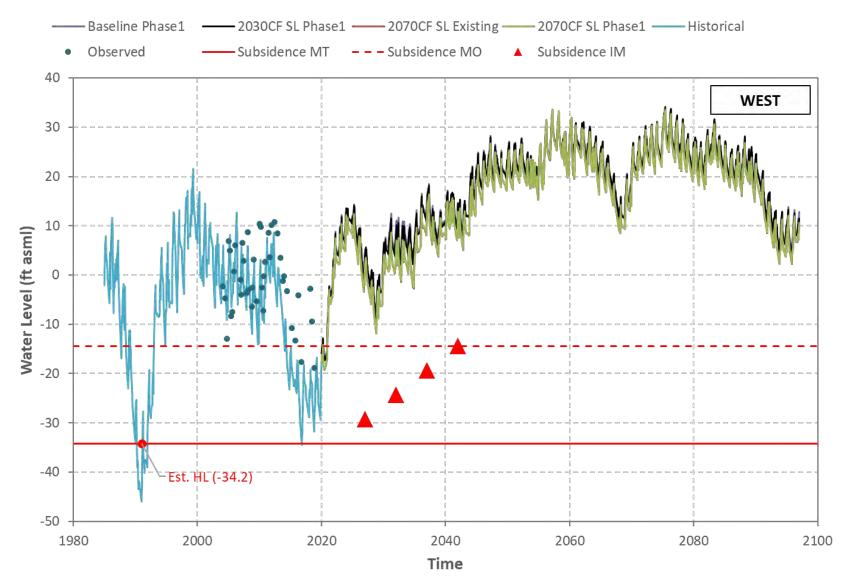
Figure I-12 Hueneme Aquifer - Simulated/Observed Water Level (Well 02N23W13K03S).
