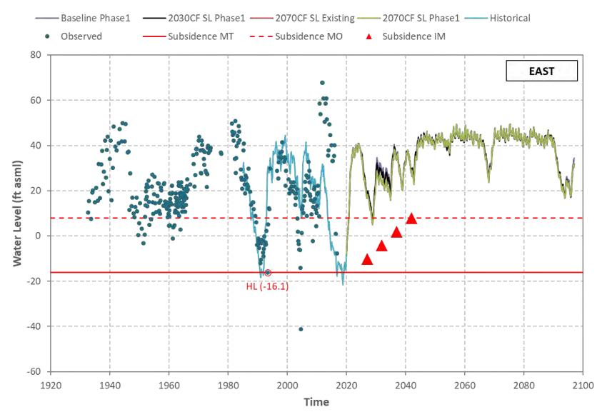
Figure I-17 Mugu Aquifer - Simulated/Observed Water Level (Well 02N22W08P01S).
