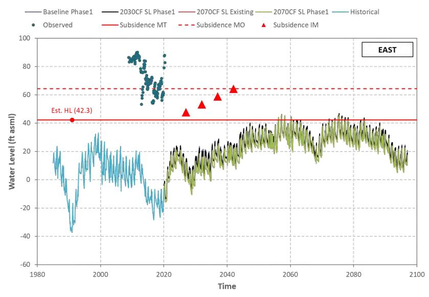
Figure I-5 Hueneme Aquifer - Simulated/Observed Water Level (Well 02N22W09L04S).
