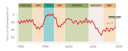
Figure 3. Example seasonality and interannual variability in depth-to-groundwater over time. Selecting one point in time, Spring 2018, such as to characterize groundwater conditions in GDEs fails to capture what groundwater conditions are necessary to maintain the ecosystem status into the future so adverse impacts are avoided.
