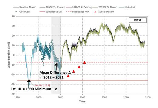
There were two exceptions to this HL estimation method, the Mugu wells 02N22W08G01S and 02N22W19M04S (Figures I-16 and I-20, respectively). For these wells, the estimated HL using modeled GWL ended up being higher than the observed HL measurement near 2020, so the HL near 2020 was used instead.
