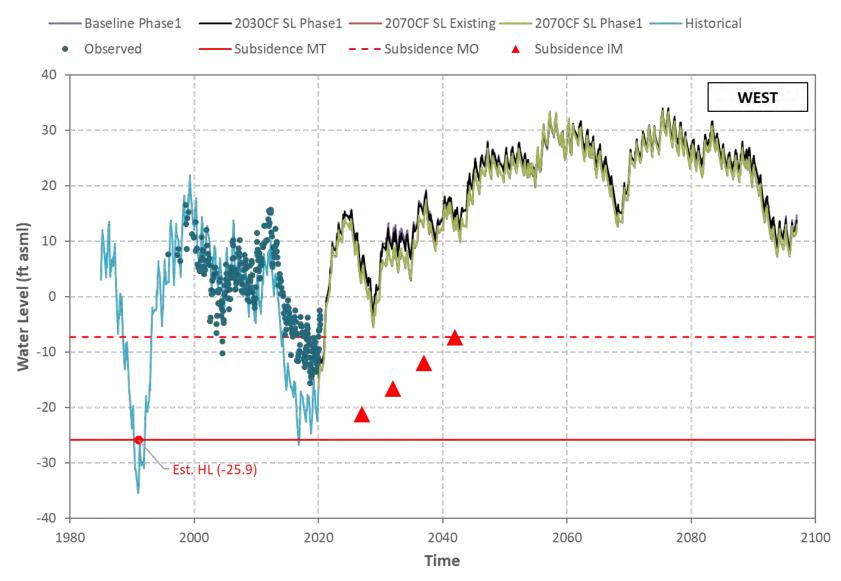
Figure I-14 Hueneme Aquifer - Simulated/Observed Water Level (Well 02N23W15J01S).
