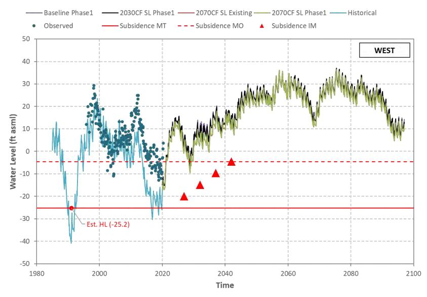
Figure I-9 Hueneme Aquifer - Simulated/Observed Water Level (Well 02N22W07M01S).
