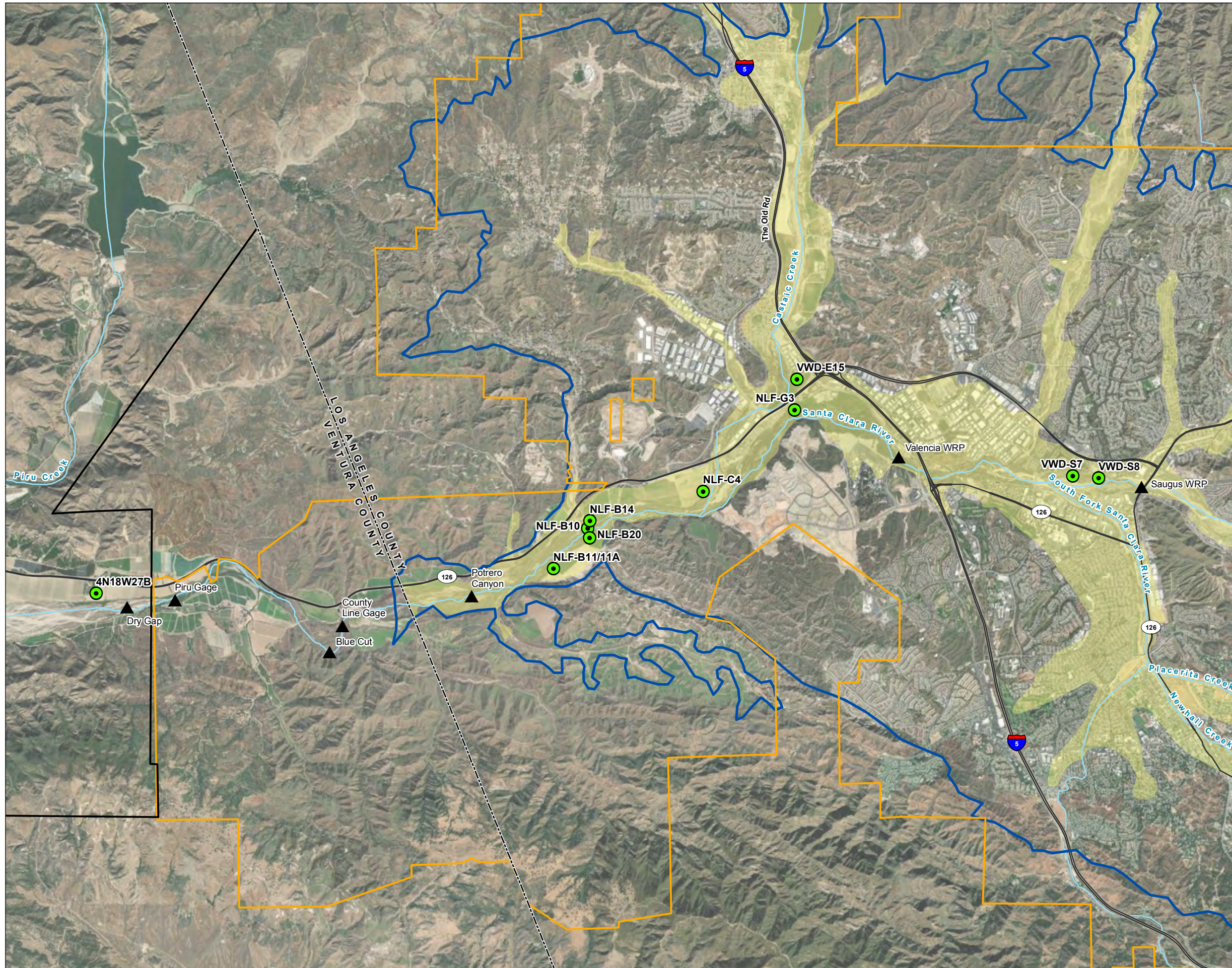
FIGURE 5-34 Wells Used for Evaluating Groundwater-Surface Water Interactions Santa Clara River Valley East Groundwater Subbasin Groundwater Sustainability Plan
