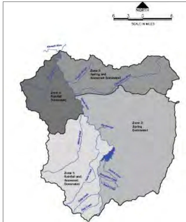
FIGURE 2. HYDROLOGICAL ZONES IN THE SHASTA BASIN BASED ON THE DOMINANT HYDROGRAPH COMPONENTS THAT DETERMINE RUNOFF PATTERNS IN THE MAINSTEM SHASTA RIVER. BOUNDARIES ARE APPROXIMATE. GRAPHIC FROM: (Mcbain & Trush, Inc et al. 2010).
