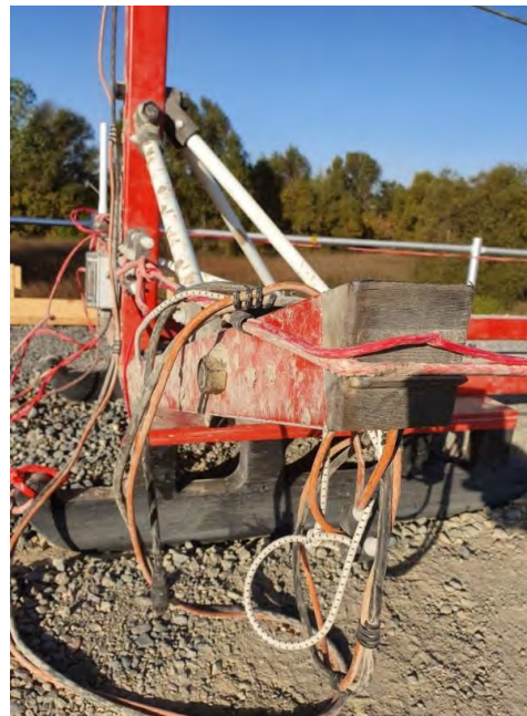
Figure A2- 2 Close-up photo showing the transmitter frame mounted on the sled
