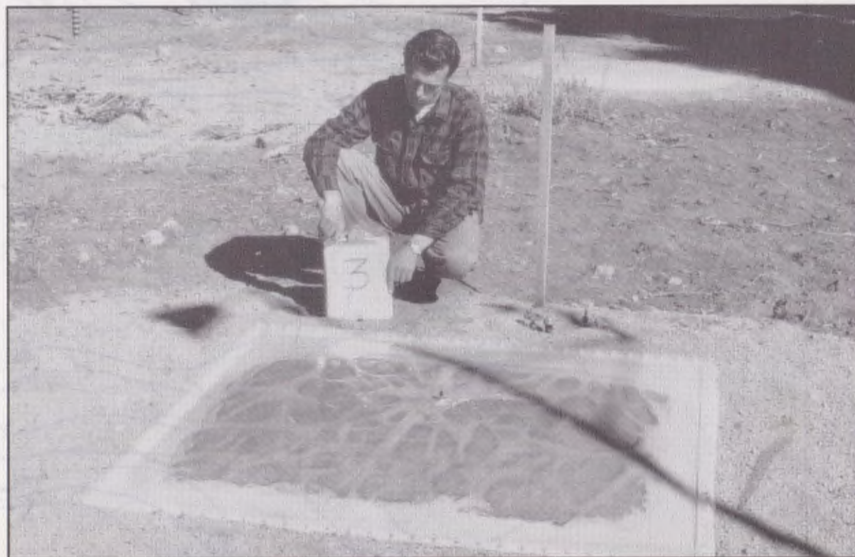
Remote sensing of data is now being used to augment manual measurement of snow courses. This snow pillow, filled with an antifreeze mixture, will provide data to be telemetered to a remote computer system.
