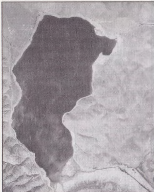
A high-altitude aerial photograph of Topaz Lake, the site of the former Alkali Lake. Water is diverted into Topaz at the bottom right of the photo, and is returned to the West Walker via the tunnel and canal visible at the upper right of the reservoir.
