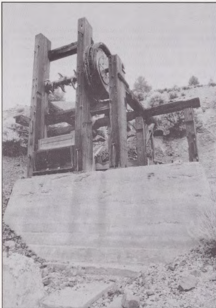
The remains of a stamp mill at Pine Grove. The large wooden wheel was turned by a belt connected to a shaft powered by steam or water. The rotation of the wheel would lift the stamps to crush the ore. The stamps have been removed from this mill, but their crankshaft remains.
