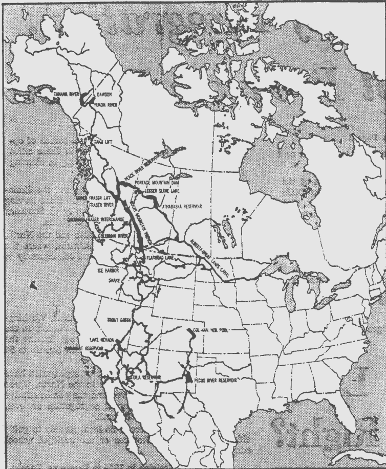
How NAWAPA Water System Would Feed Three Nations ... key to the project is the Rocky Mountain trench
