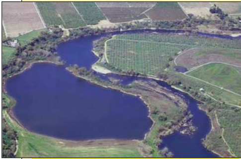
A recent restoration project recreated the original Tuolumne River channel by filling in an inchannel gravel mining pit called Special Run Pool 9, pictured here in the lower right corner; and plugging the hole between the river and the big offchannel mine pit to the left.
