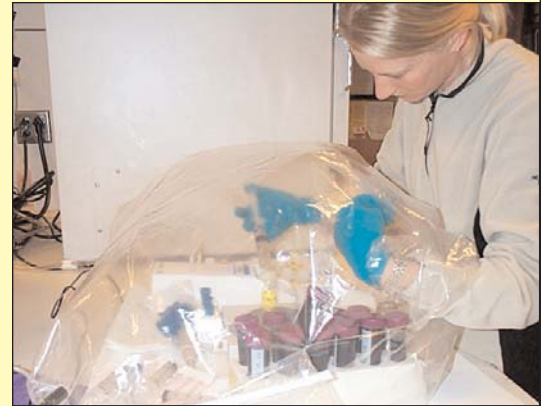
USGS's Jennifer Agee sampling sediment in an anoxic glove bag. Photo: Mark Marvin-DiPasquale
