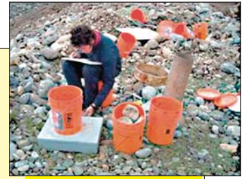
Joshua Weinstein of URS separates largest dredger material at Merced River Ranch.
