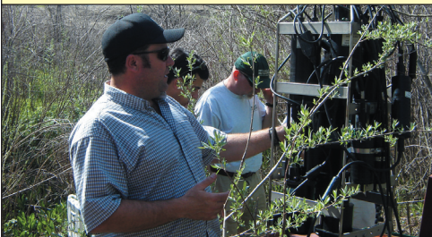
USGS scientists preparing to deploy an optical instrument package in a tributary of the Sacramento River. Once deployed in several meters of water, such instruments are programmed to come to life every 15 minutes — firing off a burst of sound to measure currents and turbidity, shining a bright light to catch refractions off particles floating around, and sucking water through various sensors to measure glow and light absorption. Pictured here: Bryan Downing, Brian Pellerin and Brian Bergamaschi.
