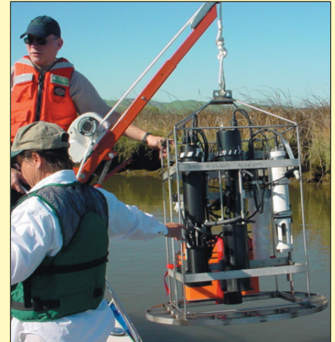
USGS's Brian Bergamaschi and Gail Wheeler lowering hydro-optic instruments into a tidal slough on Browns Island.
