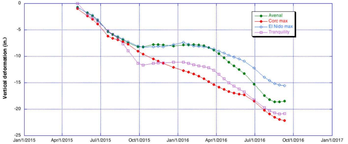
Figure 5-115. Recent Land Subsidence at Key San Joaquin Valley Locations (Source: Progress Report: Subsidence in California, March 2015 – September 2016 , Farr et. al. JPL, 2017)
