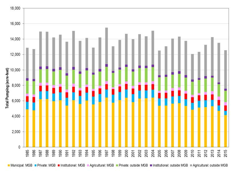
Figure 12. Simulated Groundwater Pumping by Use Type and Location
