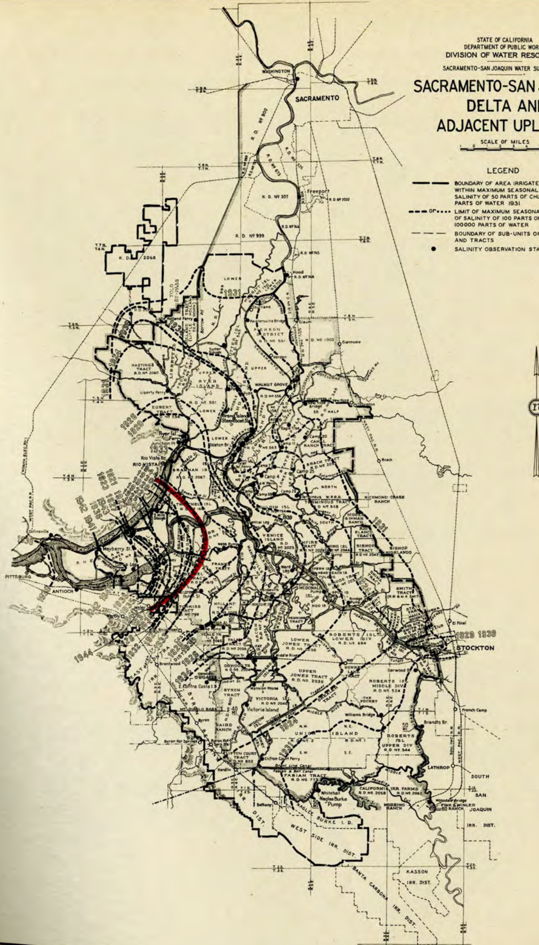
MAXIMUM SEASONAL SALINITY ENCRAGEMENT OF 100 PARTS OF CHLORINE PER 100,000 PARTS OF WATER, SACRAMENTO-SAN JOAQUIN DELTA 1920-1944
