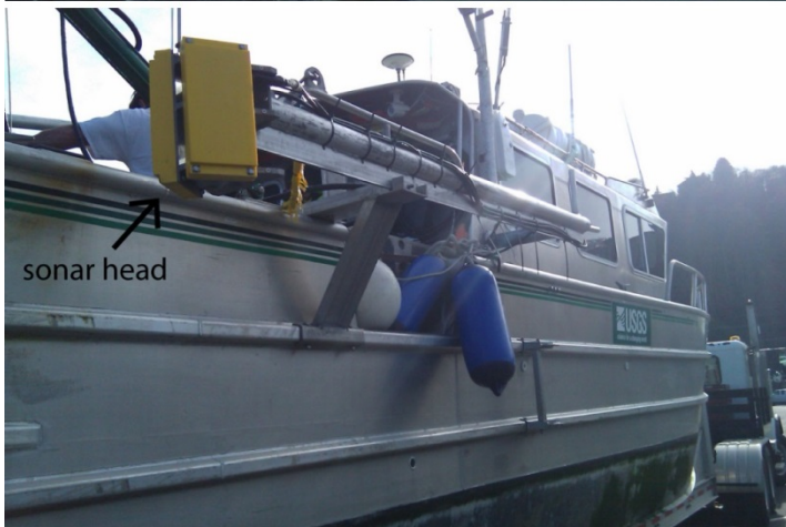
Figure 3. Fore and aft views of the SWATHplus sonar pole mount on the U.S. Geological Survey Pacific Coastal and Marine Science Center R/V Parke Snavelly .
