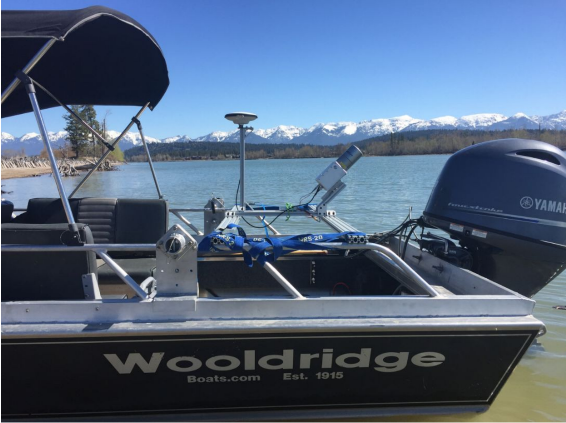
Figure 26. A photograph of the LiDAR scanner and GPS unit mounted in our jet boat.
