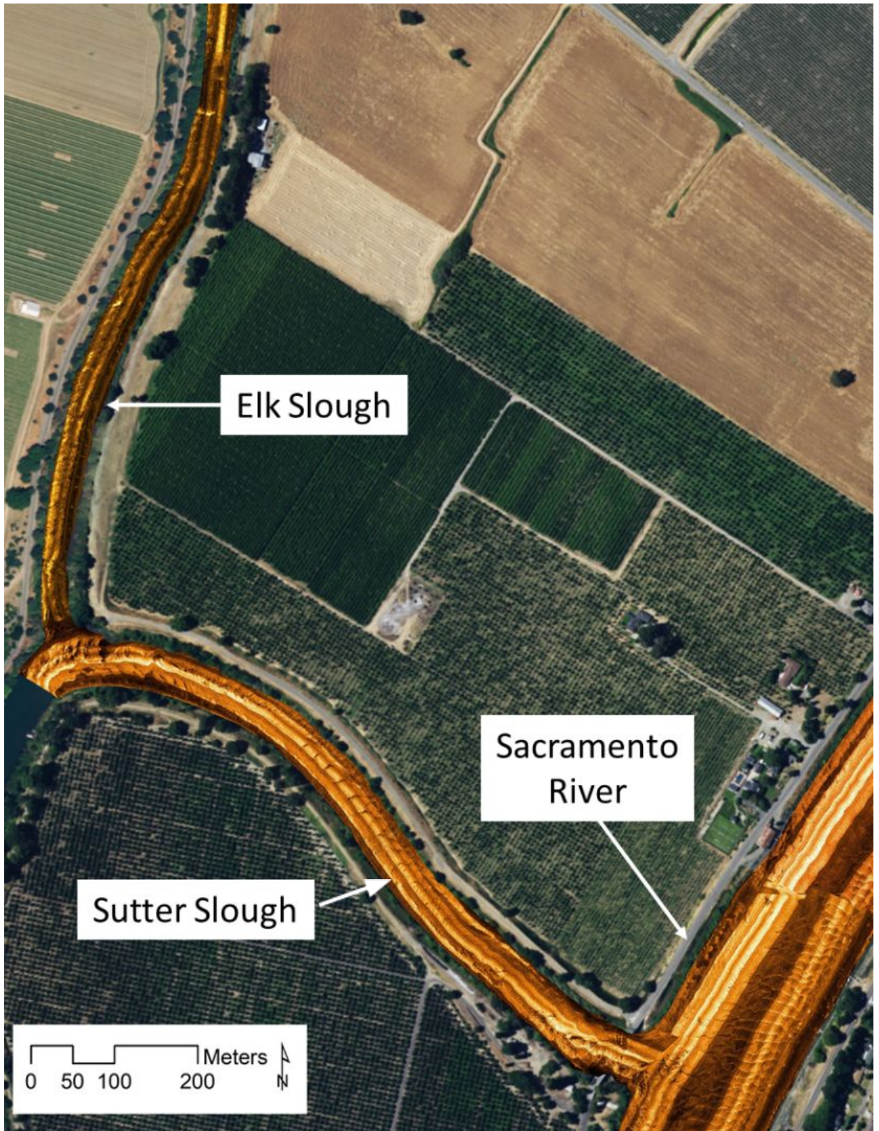
Figure 12. An example of sonar Tiff images of Elk Slough, Sutter Slough and the Sacramento River displayed against the 2016 NAIP imagery. Note the complexity of the channel bottom in these areas due to how river flow transports and deposits sediment creating different bed forms and the impacts to those processes due to bridge piers and confluence zones of sloughs and the river.
