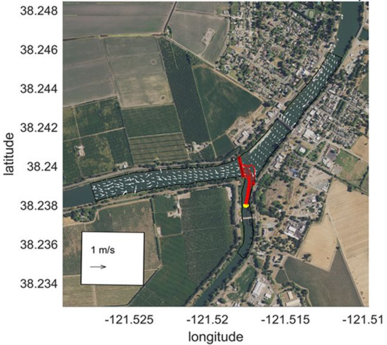
Figure 43. A plot of surface water drift paths (red arrows) relative to the flow vectors (white arrows) for the Sacramento River near Georgiana Slough. Note that the flow vectors above Georgiana Slough are pointing downstream while the flow vectors below Georgiana Slough are both chaotic and pointing upstream. The tide shifted from slack to flood tide at the time data was collected in this location.
