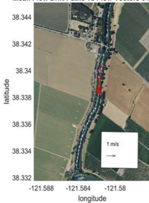
Figure 54. A plot of drift paths (red arrows) relative to the flow vectors (white arrows) for the bottom segment of Elk Slough.
