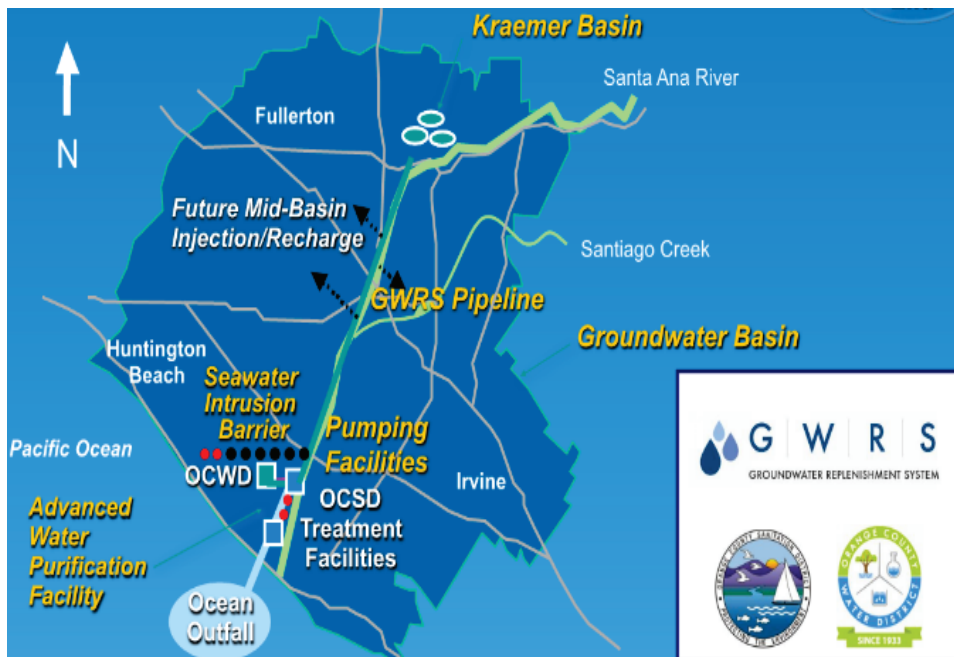
Figure A.2-2. Map of GWRS facilities, pipeline and recharge basins (Source: GWRS)
