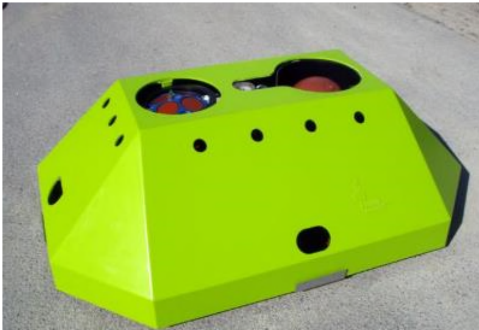
Figure C-5. Trawl and Debris Resistant ADCP Platform with Acoustic Pop-up Buoy
