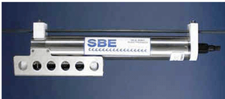
Figure A-3. Seabird MicroCAT SBE-37
