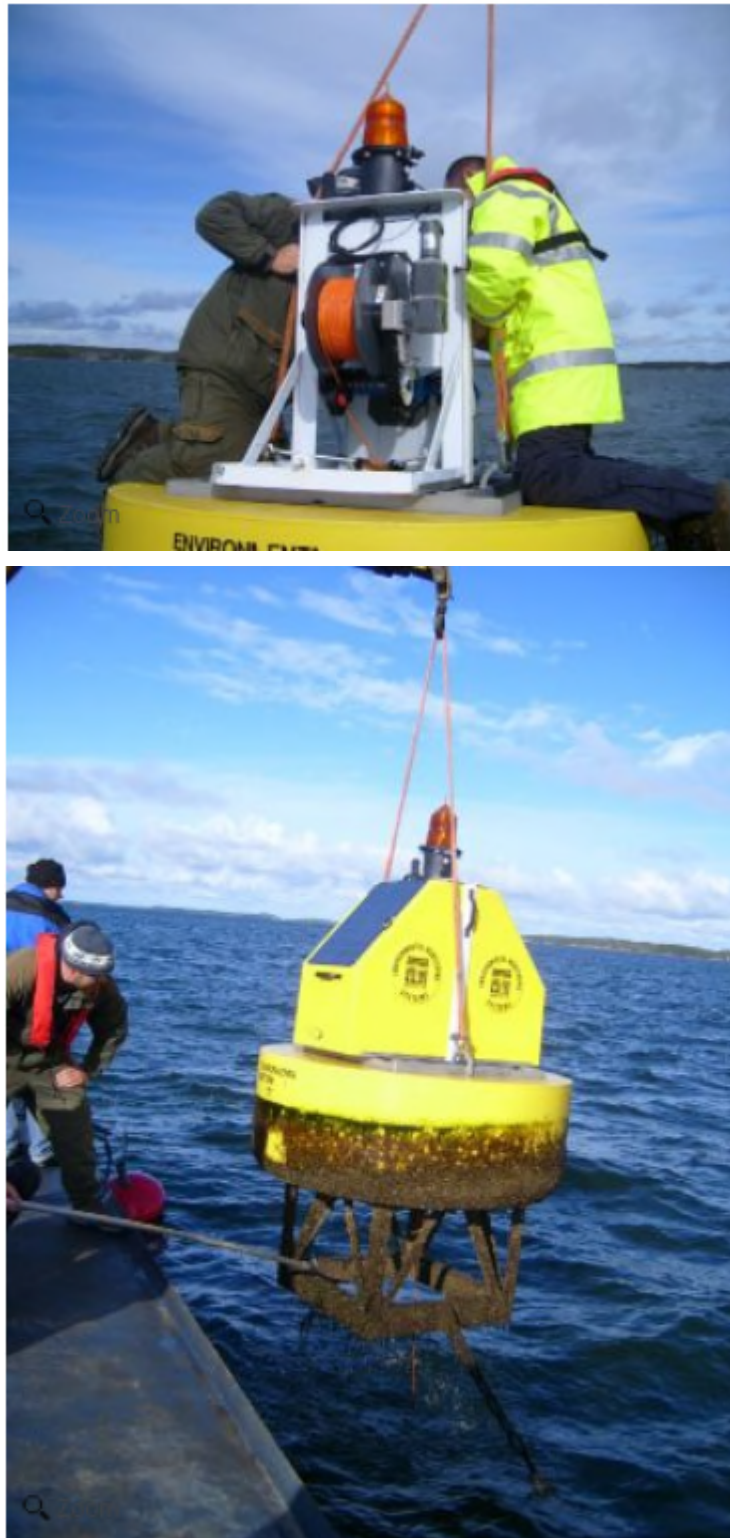
Figure C-8 YSI Buoy Vertical Profiling System
