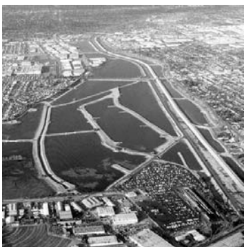
Recycled water, river water, and imported water feed the Rio Hondo Spreading Grounds to replenish groundwater in Los Angeles County. This indirect potable reuse has been practiced by the County Sanitation Districts of Los Angeles County since 1962.
