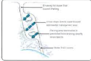
Figure 3B-2. Stormwater Runoff from Launch Parking
